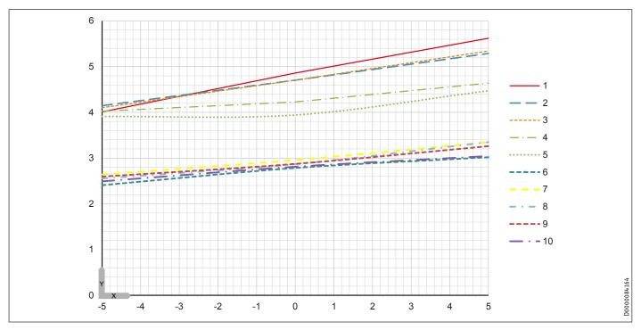
X Temperature of heat source system [°C]Y Coefficient of performance (COP)
