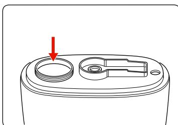
3. Pour cool, clean water directly into the tank. Do not pour anything but water into the tank.
