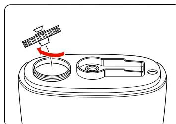
4. Close the tank lid, turning it to the right. It is important to FIRMLY secure cap after filling the tank with water.
